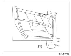
Each front door has a courtesy light (1) on its inside bottom. It lights automatically when the door is opened.
